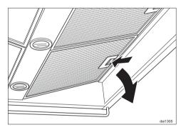
■ To remove the grease filters press the locking clips in towards the middle of the filter. Holding carefully, lower and remove the filter.
